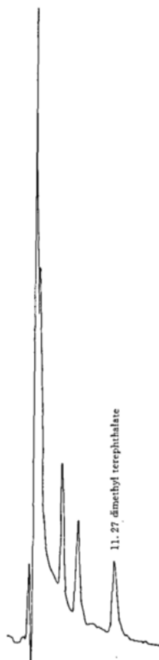
Fig. A1 Liquid chromatogram of dimethyl terephthalate standard
